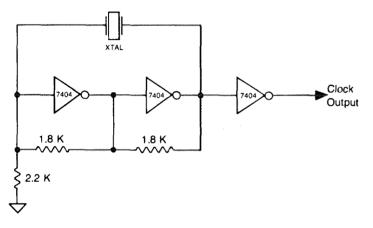
Figure 1 BASIC CRYSTAL OSCILLATOR CIRCUIT
