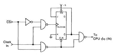
Figure 3 CLOCK STRETCHING CIRCUIT
