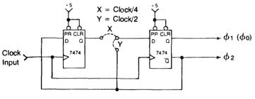
Figure 2 DIVIDER/TWO PHASE CIRCUIT
