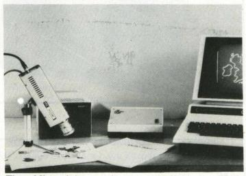
The Microsight package comprises a CCTV camera, Microeye interface and software.
