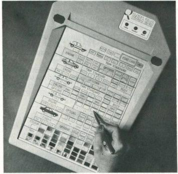
The QCSL Data Tab, a plug-in electronic data pad.
