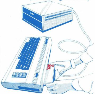
The IEEE 488 is probably the most powerful and flexible of all interfaces and at DAMS we have now harnessed it into a special cartridge, which plugs easily into the back of your VIC 20 or Commodore 64 computer, allowing for the connection of all peripherals previously associated with the PET range to the VIC!
