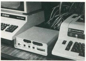
The QCSL Printerlink, a plug-in unit designed to add memory between computer/word processor and printer.
