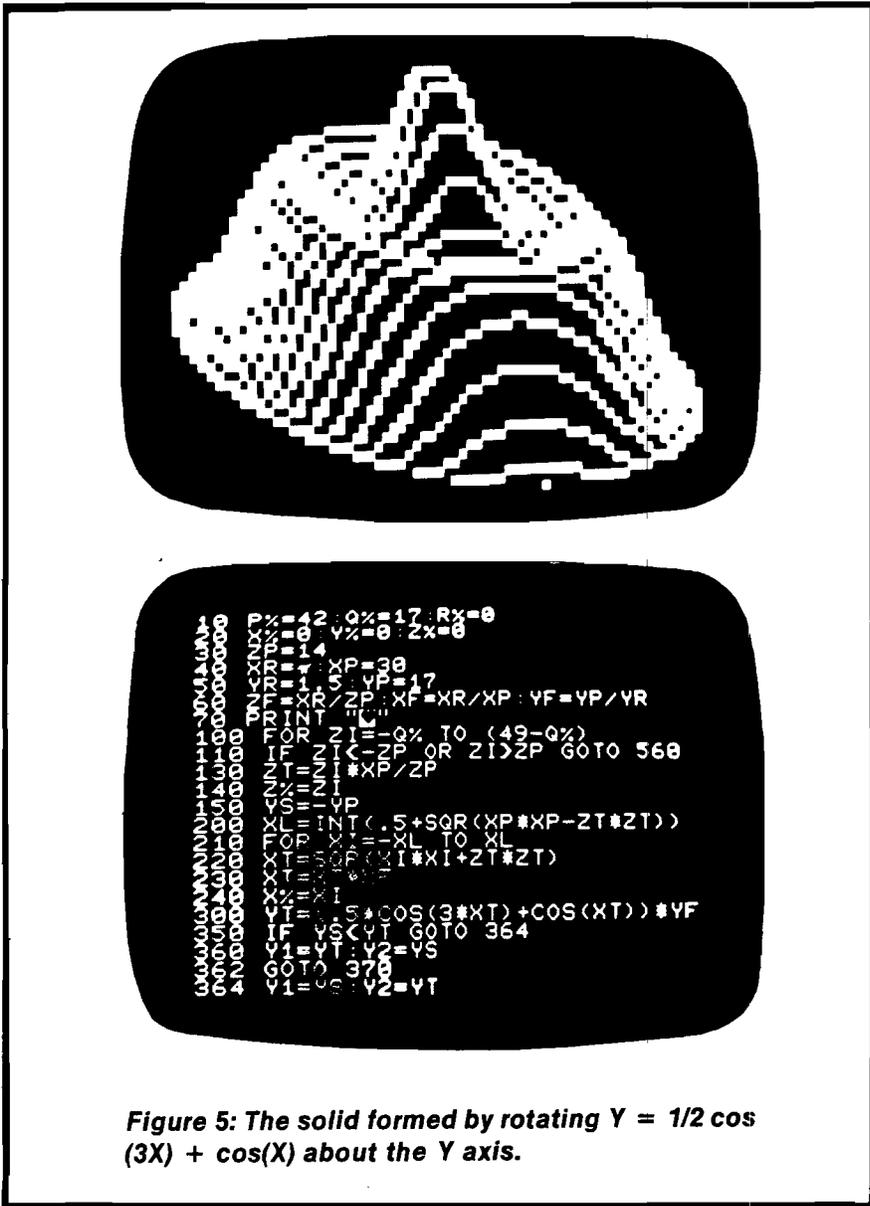
**Figure 5: The solid formed by rotating  $Y = 1/2 \cos(3X) + \cos(X)$  about the Y axis.**
