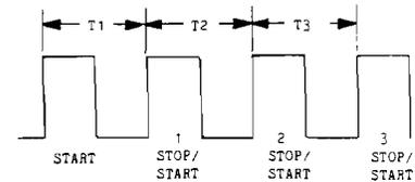
This article will use the SYM-1 board's 6532 timer and keyboard display to create a device which can measure up to 50 time intervals, store them in memory and then read them out one at a time.
