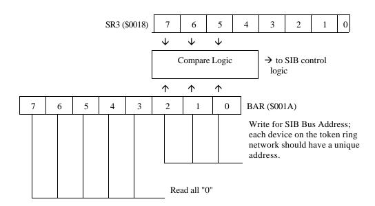
Figure 1-15 Bus Address Register (BAR)
