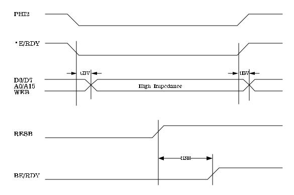
Figure 3-4 AC Timing Diagram #4
