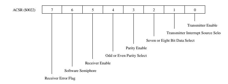
Figure 1-9 ACSR Bit Assignments
