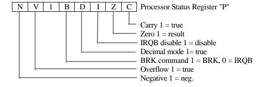
Figure 1-17 W65C02S Status Register Coding
