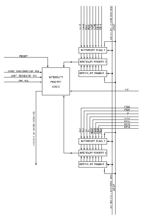
Figure 5-2 W65C134S Interrupt Controller Block Diagram
