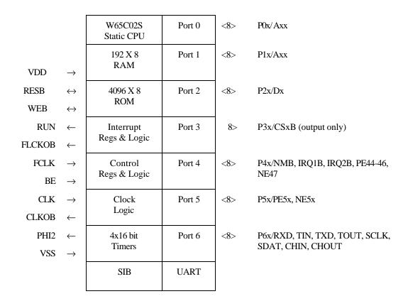
Figure 2-1 W65C134S Interface Diagram
