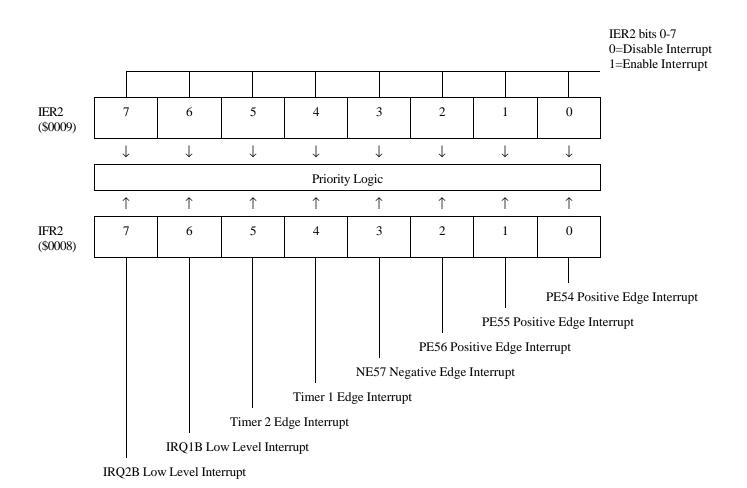
Figure 1-6 Interrupt Enable Register Two (IER2) (\$0009) and Interrupt Flag Register Two (IFR2) (\$0008)
