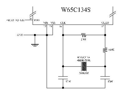
Figure 5-9 W65C134S Resonator Circuit
