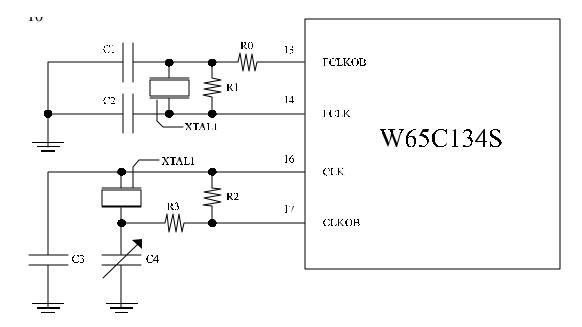
Figure 5-7 Oscillator Circuit
