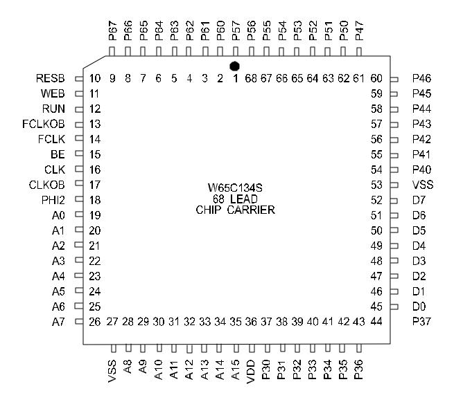
Figure 2-2 W65C134S 68 Lead Chip Carrier Pinout
