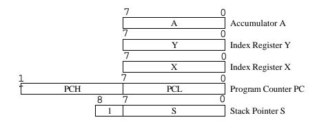
Figure 1-16 W65C02S Microprocessor Programming Model
