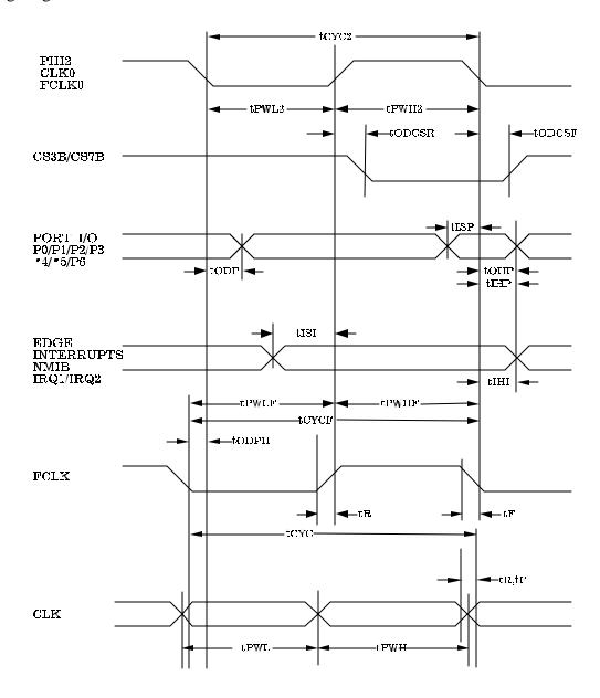
Figure 3-1 AC Timing Diagram #1
