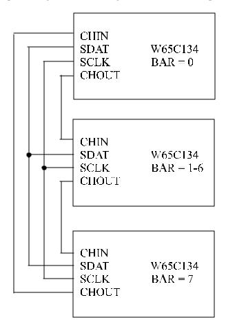
Figure 1-14 W65C134S Serial Interface Bus (SIB) Wiring Diagram
