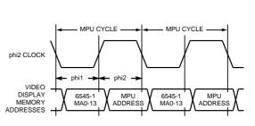
Figure 6. phi1/phi2 Interleaving
