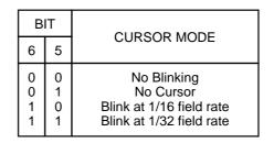
Note that the ability to program both the start and end scan line for cursor enables either block cursor or underline to be accommodated. Registers R14 and R15 are used to control the character position of the cursor over the entire 16K address field.
