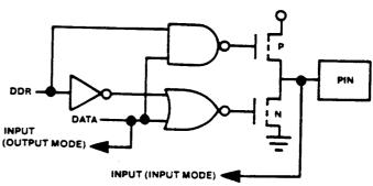
Figure 14. Port A Buffer Circuit (PA0-PA7)
